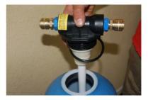
4 Reconnect the bottle to the machine; ensure that the inlet port goes into the left-hand side port on the machine.
