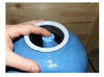
9 Once the riser tube is centrally positioned into the empty vessel, start to fill the vessel with mixed bed resin. A cut down funnel is a useful tool to assist filling. Fill the vessel up to the shoulder position, as indicated. Shake the container frequently to ensure a good settlement and compaction of resin. Do not overfill and ensure that the riser tube remains central during the procedure.
