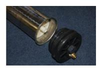
Grasp the central spigot with a pair of pliers and pull gently, turning membrane as necessary and withdraw the membrane fully from the housing.
