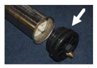
Refit pair of "C" clamps, ensuring outer lip grips the recess in the plastic end cap and the other fits over the stainless steel lip at the end of the membrane housing.
