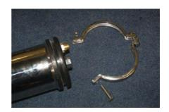
Tighten bots equally, so that a similar gap is on either side of the housing.
