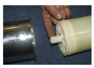
Note: insert new membrane in direction of flow arrow.
