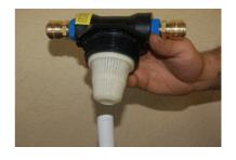
Cover the end of the tube with some sticky tape to ensure that resin does not pass down the tube whilst filing.
