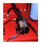
The electrical connections can be easily pulled apart. But, when reconnecting, please ensure that only the round fittings go together, and the flat fittings go together i.e. positive – orange/red and negative – black.
