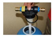
Reconnect the bottle to the machine; ensure that the inlet port goes into the left-hand side port on the machine.
