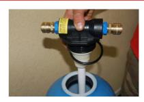
The riser tube can be slowly lifted out whilst shaking the blue vessel and you must inspect this tube to ensure that the white plastic distributors at the top and bottom are intact and undamaged. Again at this time ensure that the black rubber "O" ring is safe.
