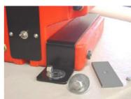
In Line Fuse Holder with Fuse (40Amp)
